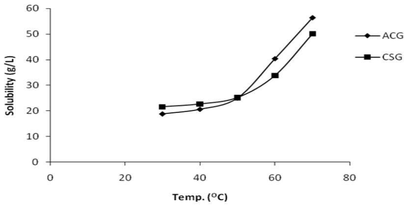
Figure 2: Graph of solubility of paracetamol in 1 %w/v gum solution versus temperature
