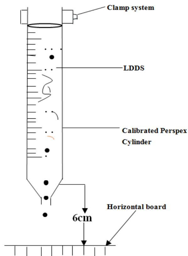
Figure 1: Schematic diagram of system for determining time, t, for syrup to fall under gravity.
